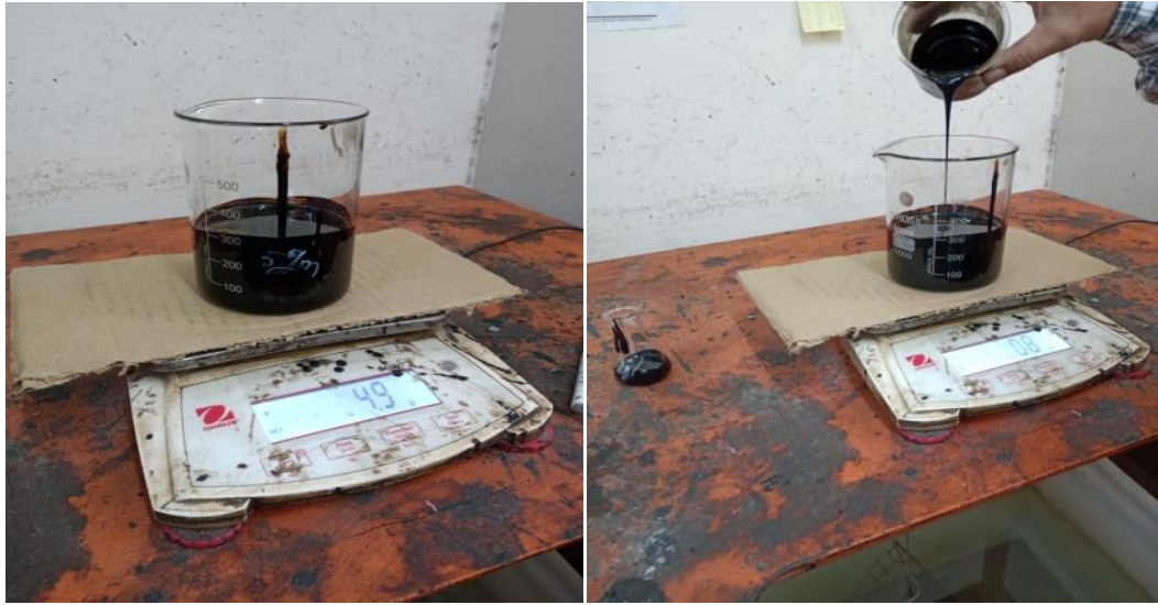
Photo-9: Bitumen and addition of Bottom Residue
