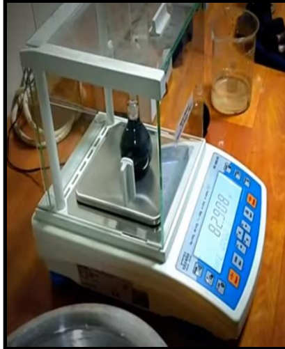
Photo-2: Specific gravity testing of bitumen
