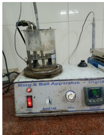
Photo-6: Softening point testing of bitumen
