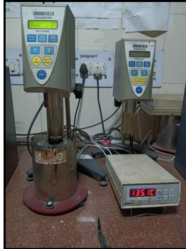
Photo-5: Viscosity testing of bitumen
