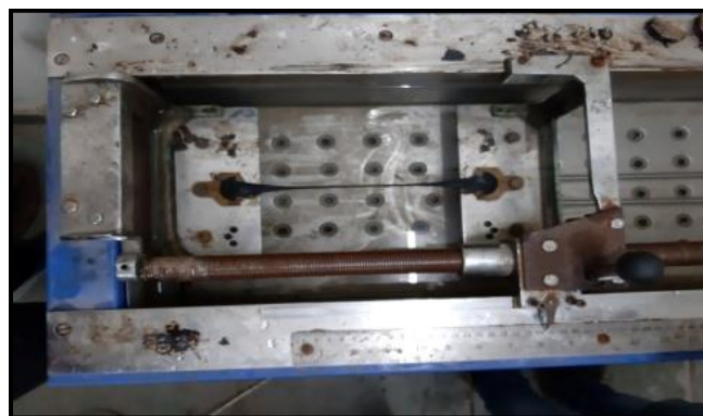
Photo-4: Ductility testing of bitumen
