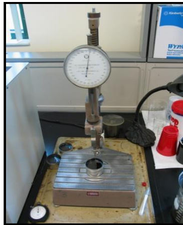
Photo-3: Penetration testing of bitumen
