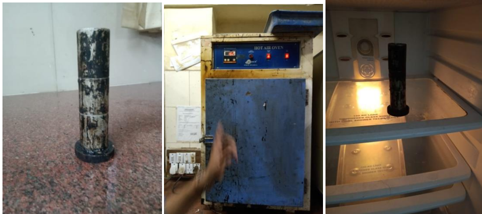
Photo-11: Separation Test Set up
